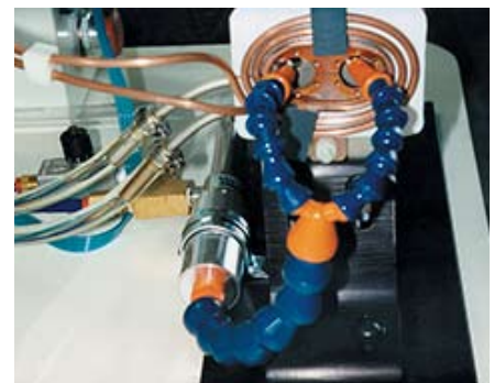
A Model 3215 Vortex Tube cools a die on a medical tube forming machine.
