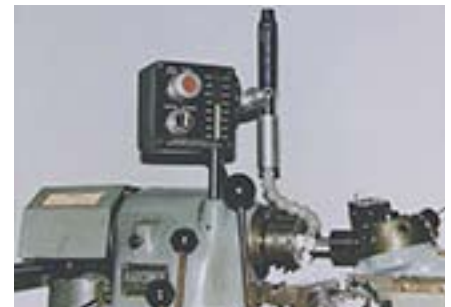
The Adjustable Spot Cooler maintains critical tolerances on machined plastic parts.
