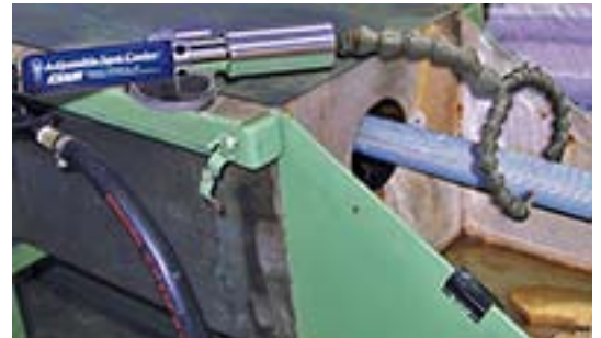
PVC hose is cooled at the exit of an extruder so it can be coiled immediately.
