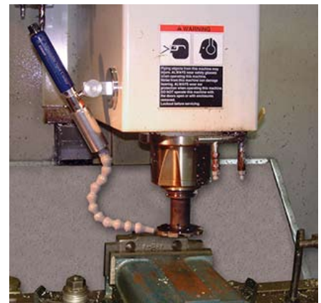
The Adjustable Spot Cooler replaces flood coolant and eliminates
